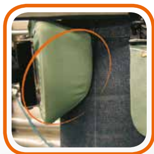
Stiro tasche/patella vaporizzante Pocket/Flap pressing device, heated by steam and steaming
