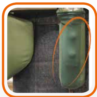
Stiro tasche/patella vaporizzante Pocket/Flap pressing device, heated by steam and steaming
